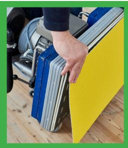
**9** During the last sanding cycle, we used our useit® Superpad P with a grain of 120 to prepare the flooring for the next work
