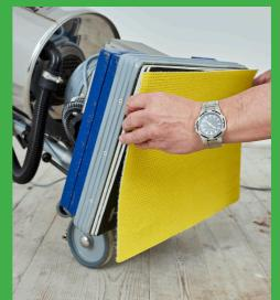
5 Here comes the first important step of our floor renovation process! Removing the dirt layer using a sanding pad in grain size 40.
