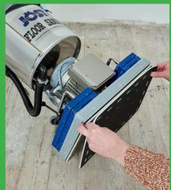
**4** The adapter pad is used to adapt to the unevenness of the flooring – it's positioned on the machine using Velcro.
