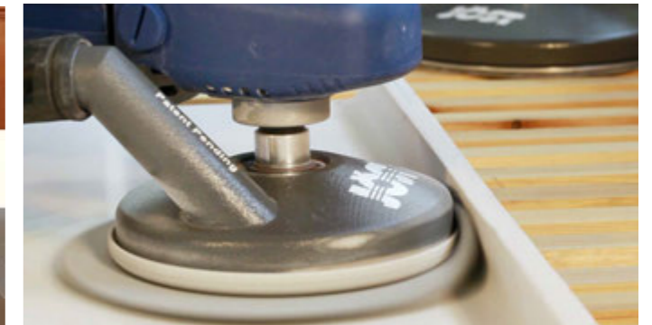
Sanding of chamfered edges with P1 dust-free sanding system
