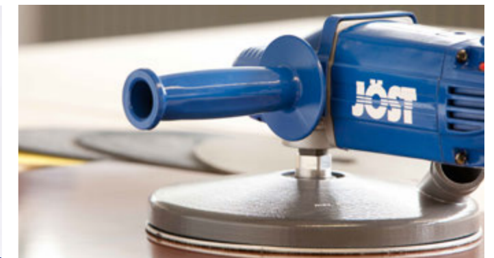
Surface grinding of a glue line with P220
