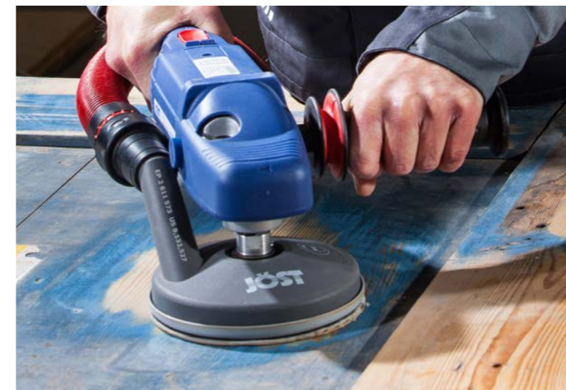
Application example paint removal with the P1 dust-free sanding system and useit®-Abrafilm®
